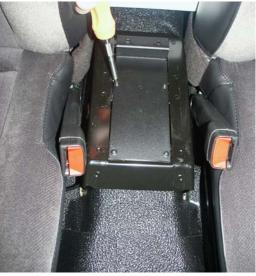
Attach rear extrusion bracket (CM001380) to vehicle using factory screws from, "partial console," removal.
